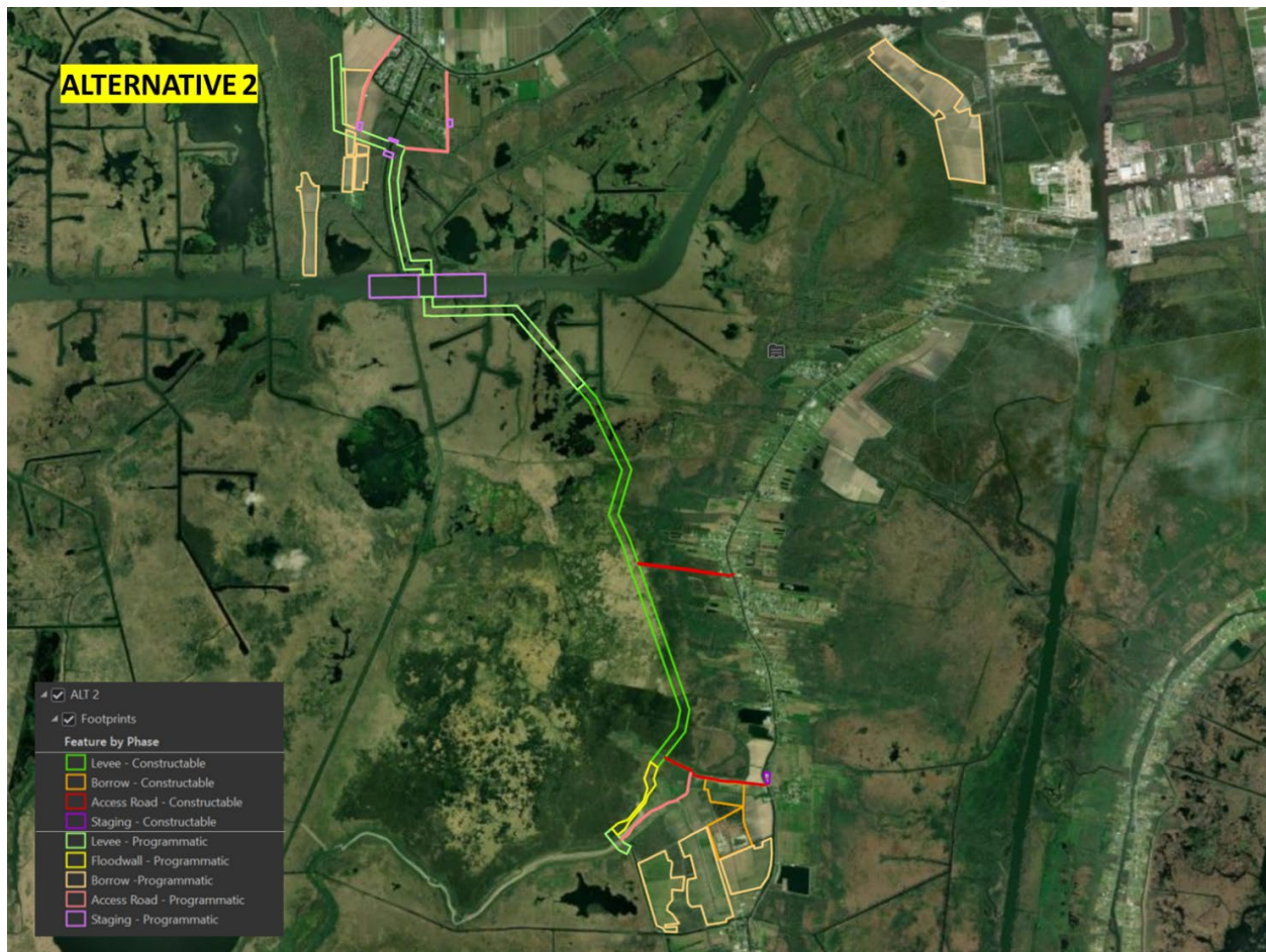
Figure 4: Reach A alternative 2 with potential borrow, structures, haul routes and mitigation.
